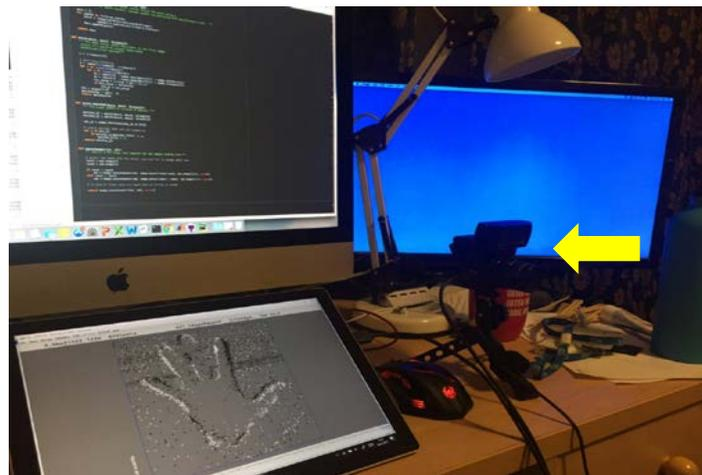
Figure 2: The use of a Dynamic Visual Sensor (arrow) with a commercial computer
