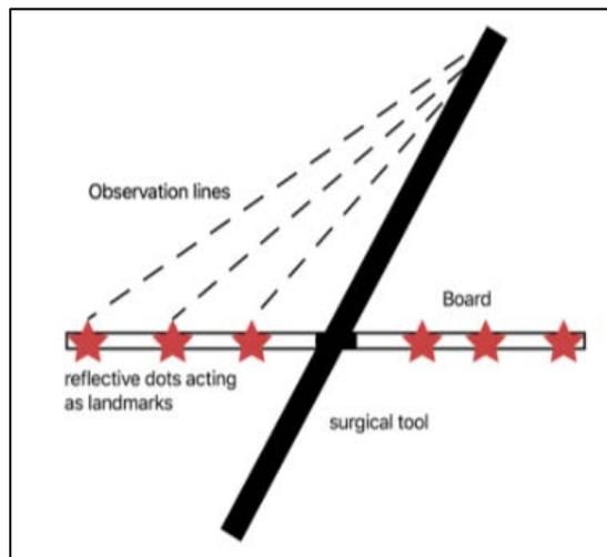
Figure 1: An illustration of how 3D mapping can be achieved by instrumenting the handle end of a laparoscopic tool.
