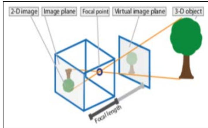
Figure 3: Pinhole camera model (15)
